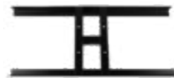
Part no. 5037 Foot for slabs for 40x40 cm concrete blocks Weight: 9,000 kg Material: Steel
